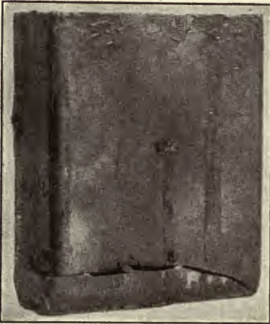
FIG. 67.—Cracked jar due to buckled plates.
