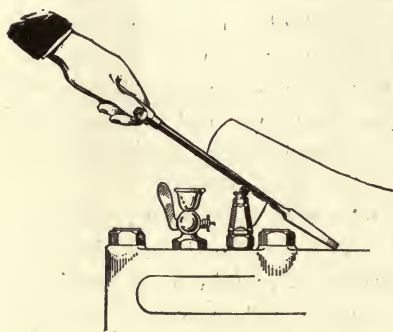
FIG. 331.—Method of locating a misfiring cylinder.
