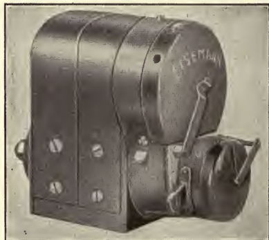
FIG 221.—Eisemann high-tension magneto, Type G4, II edition.
