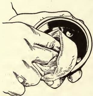
FIG. 92.—Method of cleaning distributor head.
