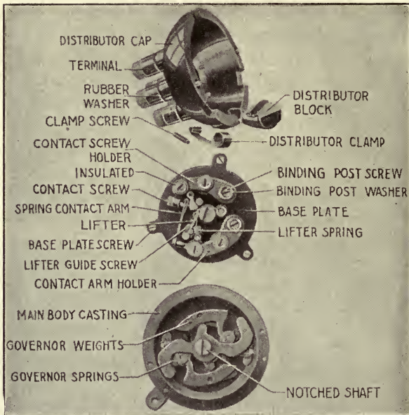
FIG. 95.—Construction of Atwater-Kent ignition unit, type K-2.
